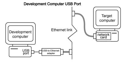
To connect the USB-to-Ethernet protocol interface hardware to the USB port on the development computer:
