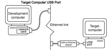
To connect the USB-to-Ethernet protocol interface hardware to the USB port on the target computer:
